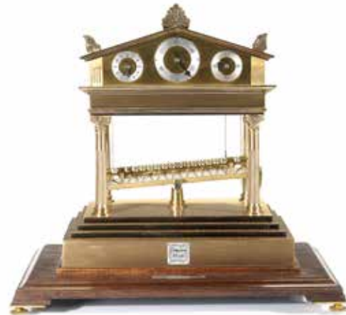
455 A LATE 20TH CENTURY BRASS ROLLING BALL TIMEPIECE Thwaites & Reed the silvered ball rolling on a tilting platform with centrally mounted bar displaying running seconds, the movement housed in the pediment and wound from the side, with glass shade, 44cms high excluding glass case £3,000 - 5,000 €3,800 - 6,400
